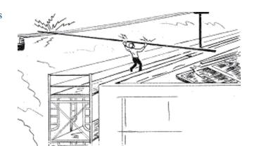
the bracket to the top of the building, he turned it to a horizontal position. In the process, the bracket came in contact with high- voltage electrical lines that were 10 feet away from the scaffold. He was electrocuted and fell 35 feet to his death.
